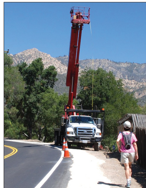
Verizon simulated the proposed cell tower height with a truck boom.
